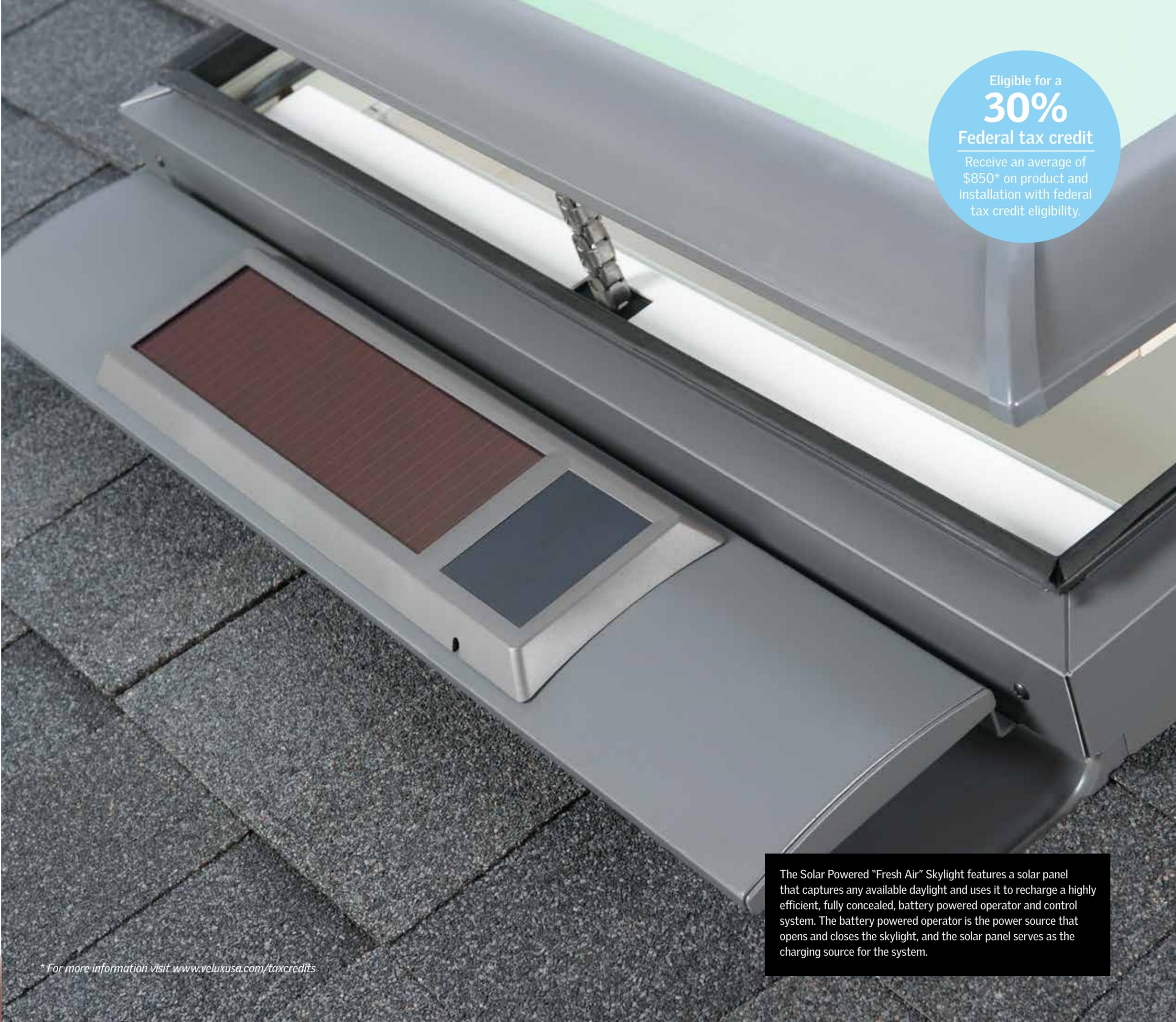
The Solar Powered "Fresh Air" Skylight features a solar panel that captures any available daylight and uses it to recharge a highly efficient, fully concealed, battery powered operator and control system. The battery powered operator is the power source that opens and closes the skylight, and the solar panel serves as the charging source for the system.
